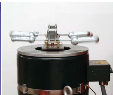
◀ RIBE® Engineering Indoor vibration test bed.
