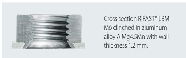
Cross section RIFAST® LBM M6 clinched in aluminum alloy AlMg4.5Mn with wall thickness 1.2 mm.
